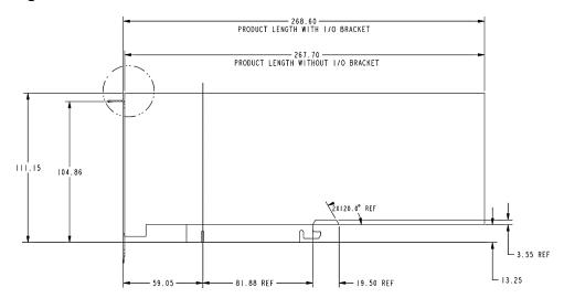
Figure 3. **NVIDIA L40S PCIe Card Dimensions**
