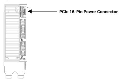
Figure 4 3 shows the pin assignments for the PCle 16-pin power connector, per PCle CEM 5.0 specification.
