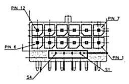
12V PWR Cable Plug Pin Assignment Signal +12 V 1 to 6 7 to 12 Ground CARD PWR STABLE CARD\_CBL\_PRES# S2 SENSE0 S3 SENSE1
